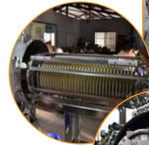
A specially designed roller cart effortlessly tilts and rolls the membrane cartridge directly into the pressure housing to ensure precise placement.
