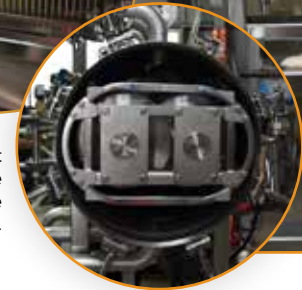
A specially designed roller cart effortlessly tilts and rolls the membrane cartridge directly into the pressure housing to ensure precise placement.
